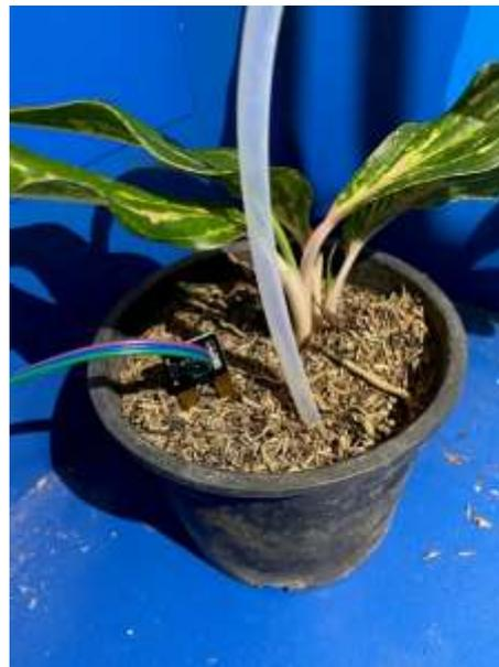
**Gambar 6.** Sensor kelembaban tanah
