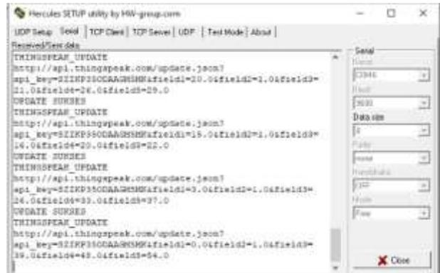
**Gambar 8.** Pengujian *upload* data ke thingspeak.com
