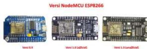
Gambar 1. Tipe Nodemcu ESP 8266 (Hidayati et al., 2018)
