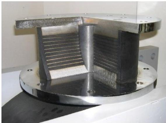
Gambar 10. LRB (*Lead Rubber Bearing*)
