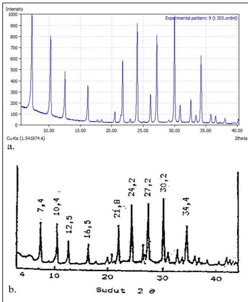
**Gambar 2.** Difraktogram Zeolit 4A (a.) Zeolit 4A Hasil Sintesis (b.) Zeolit 4A Standar [Murat dkk., 1992]
