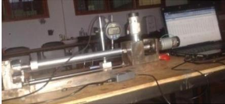
Gambar 3.4 Alat Ukur Kebulatan (*Roundness Tester Machine*)
