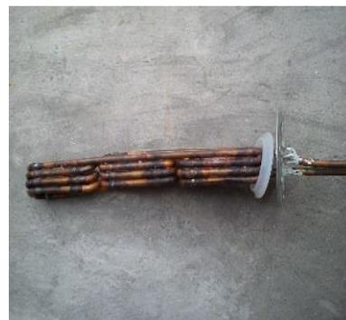
**Gambar 4.** Kondensor *Dummy* Multi *Helical Coil*
