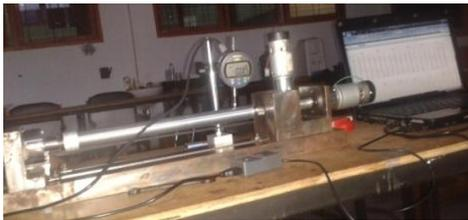
Gambar 2.3 Alat Ukur Kebulatan (*Roundness Tester Machine*)
