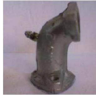
Gambar 6. *Intake Manifold* Posisi 45° (Mulyono, 2010)
