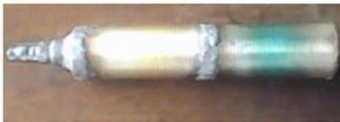
Gambar 7. *Vacuum Tube* Tipe Posh
