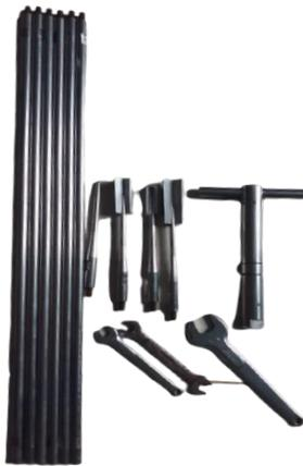
Gambar 1. Alat *Vane Shear*
