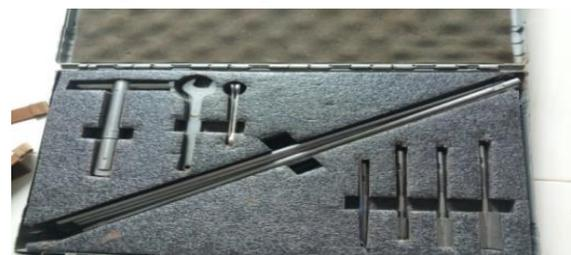
Gambar 2. Alat *Vane Shear*
