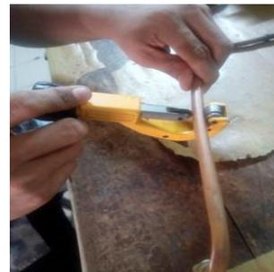
Gambar 1. Proses potong pipa
