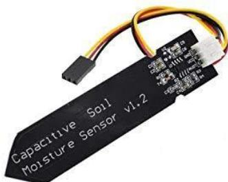
Gambar 4. *Soil Moisture Sensor*
