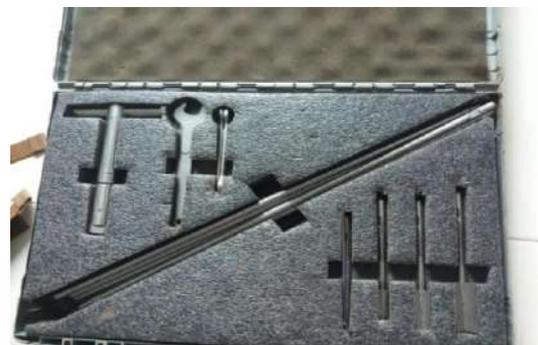
Gambar 2. *Vane Shear*
