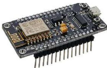
**Gambar 1.** Nodemcu ESP8266
