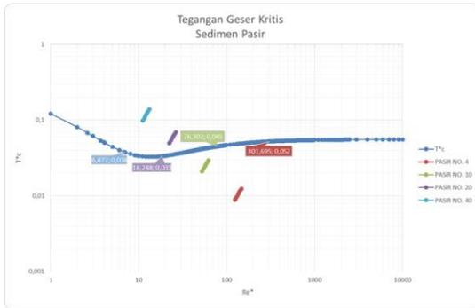
Gambar 10. Tegangan Geser Kritis Sedimen Pasir
