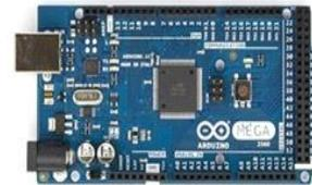
**Gambar 4.** Board Arduino Mega 2560 Tampak Depan
