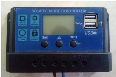
**Gambar 3.** Solar Charge Controller 10A
