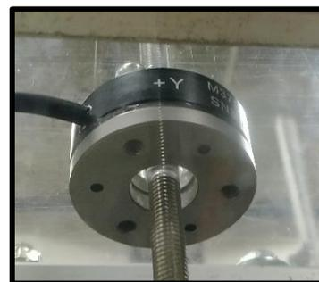
Gambar 7. Sensor *load cell*
