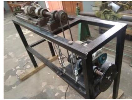
Gambar 1. *Rotary friction welding*
