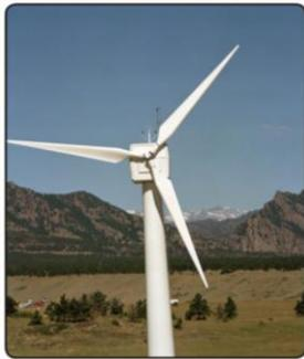
Gambar 2. Turbin Angin Sumbu Horizontal [7]
