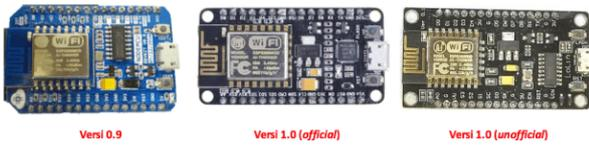
Gambar 1 Tipe Nodemcu ESP 8266 (Dewi N, 2016)
