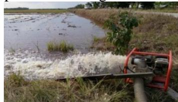
Gambar 1 Pompa *robin type RTG300FCR/LH*
