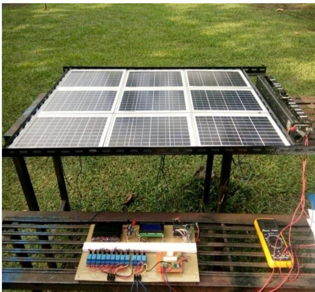
Gambar 8. Prototype PV Array 9×10 Wp
