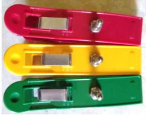
Gambar 3. Limb Clamp Electrodes
