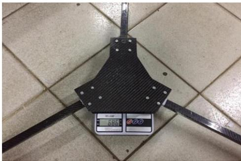
Gambar 23. Massa total rangka tricopter
