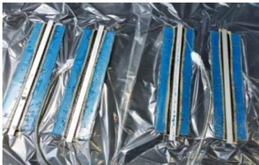
Gambar 12. Proses *Vacuum bagging*
