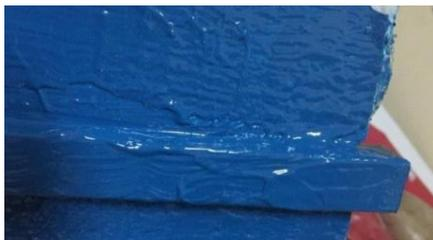
Gambar 6. Lapisan resin *gelcoat*
