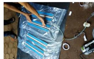
Gambar 7. Proses *vacuum bagging*
