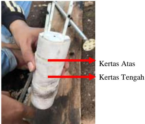
Gambar 9 Merangkai alat *groundwater velocimeter*
