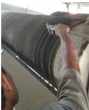
Gambar 4. Pengukuran diameter wire rope
