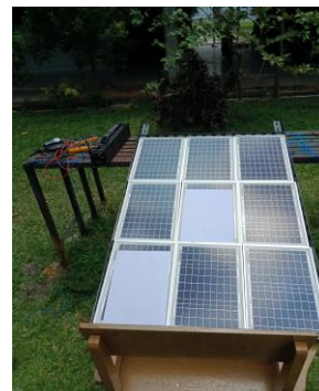
Gambar 13. Prototype PV Array 9×10 Wp Kondisi Shading 0 1 1 (22,2%)
