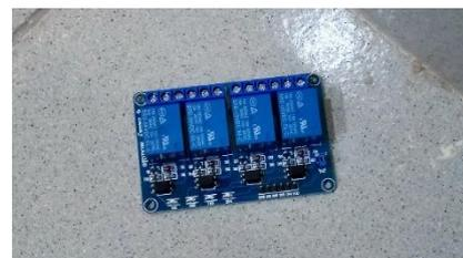
**Gambar 3.** Relay Module (4 Channel )
