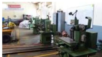
**Gambar 5.** Mesin Miling Universal ACIERA Tipe F3-10018.
