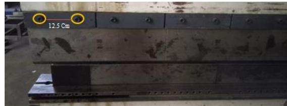
Gambar 4. Jarak antar baut 12.5 cm
