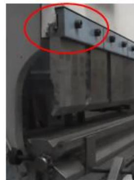
Gambar 14. Baut pencekam mesin *Press Bending*
