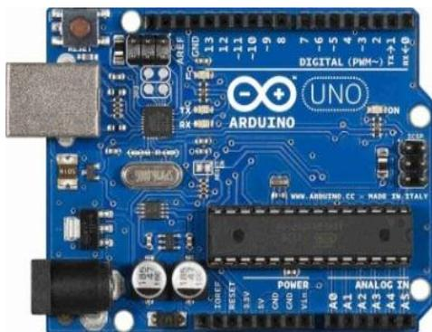
Gambar 5 Board Arduino
