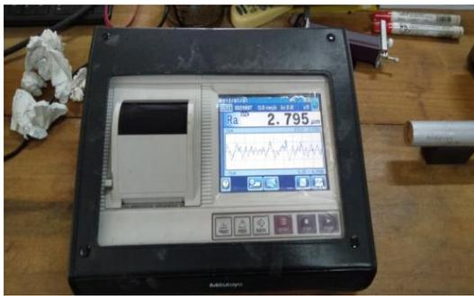
Gambar 5. Surface roughness tester
