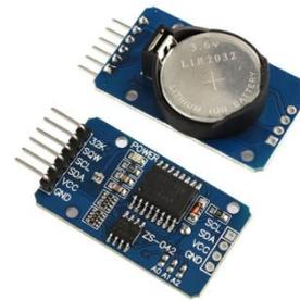
**Gambar 3.** Module RTC3231
