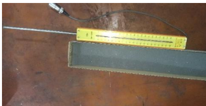
Gambar 2. Alat Linear Variable Displacement Transducer (LVDT)
