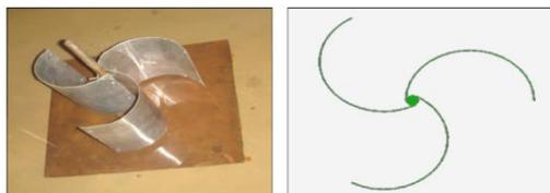
**Gambar 10.** Turbin Savonius *Single Stage Type Elliptical* Tiga Sudu
