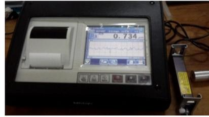
Gambar 4. Surface Roughness Tester
