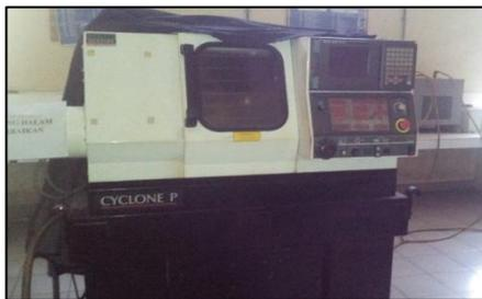
Gambar 1. Mesin CNC *Lathe Fanuc*
