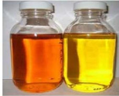
Gambar 2.2. Minyak Transformator (Sumber : PT PLN Persero 2003)
