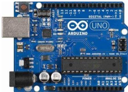
Gambar 5 Board Arduino
