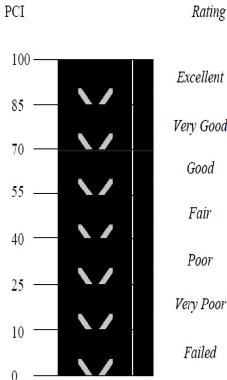
Gambar 1 Rating Kondisi Perkerasan Berdasarkan Nilai PCI
