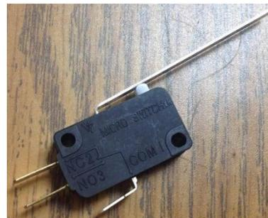
**Gambar 11. Sensor Limit Switch**
