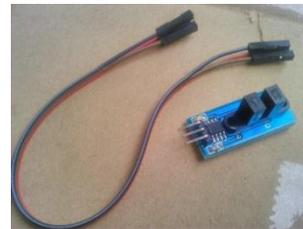
**Gambar 4.** *Photodiode* Sensor *Rotary Encoder*
