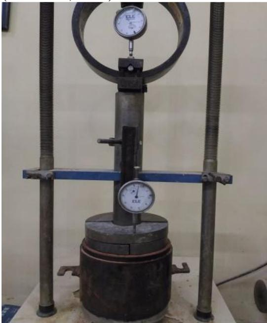
Gambar 6 Alat CBR Laboratorium
