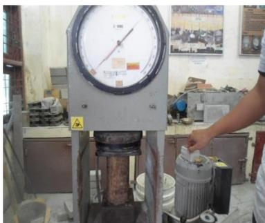
Gambar 4. Alat *Compression Test Machine*
