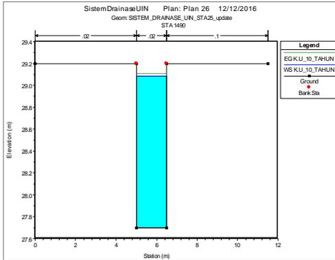
Gambar 8. Profil Penampang Drainase B3 sta 1490
