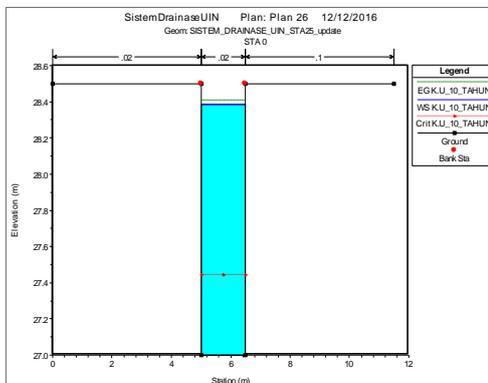
Gambar 9. Profil Penampang Drainase B3 sta 0
