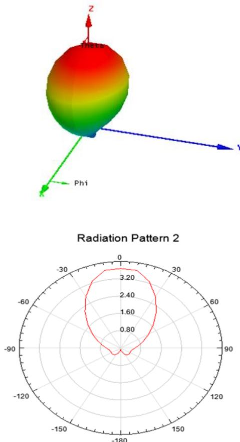
Gambar 4.3 Pola Radiasi antena
