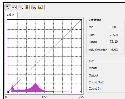
Gambar 2 Histogram Hasil Koreksi Radiometrik Band 4 Citra Landsat-7 ETM+ Perekaman Tanggal 21 November 2012
