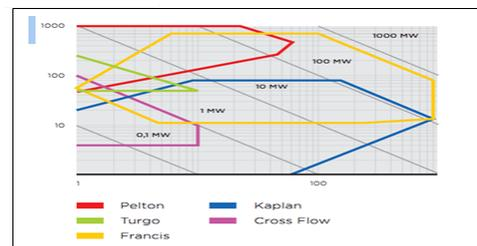
Gambar 2.3. Grafik karakteristik turbin head (m) VS flow (m<sup>3</sup>/s)
