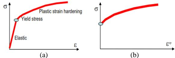
Gambar 2 (a) Kurva Tegangan Regangan Material (b) Kurva Tegangan Regangan Plastik Material yang dibutuhkan *Software* Hingga (Seismic Assessment of WSDOT Bridges with Prestressed Hollow Core Piles, 2009)
